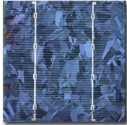
These cells are made using a process called “epitaxial growth”, whereby the crystals are grown on a flat substrate, and not cut from a large ingot.
