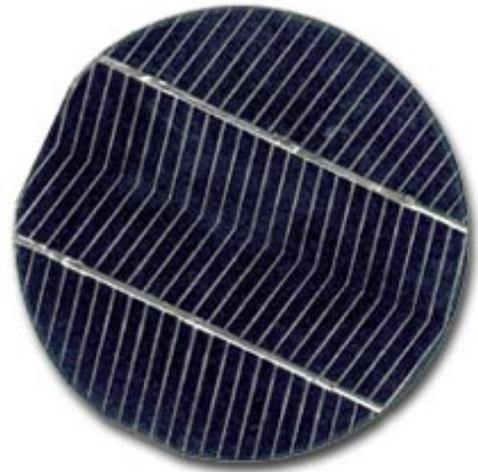
**Polycrystalline PV Cells:** Each cell is a collection of many small silicon crystals, as one can see in the photo at right. These also have pretty high efficiency (10-13%), slightly less than single crystalline cells. and very long lifetimes because the crystal structure is very stable.
